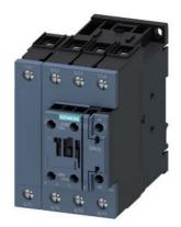
Contactor, AC-1, 60 A/400 V/40  $^{\circ}\text{C},$  S2, 4-pole, 240 V AC/50 Hz, 1 NO+1 NC, screw terminal
