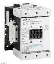
Electrically held lighting contactor, Contactor amp rating 200A, 0 N.C. / 3 N.O. Poles, 220VAC 50HZ/240VAC 60HZ coil, Non-combination type, (no disconnect device), Enclosure NEMA type (open), No enclosure
