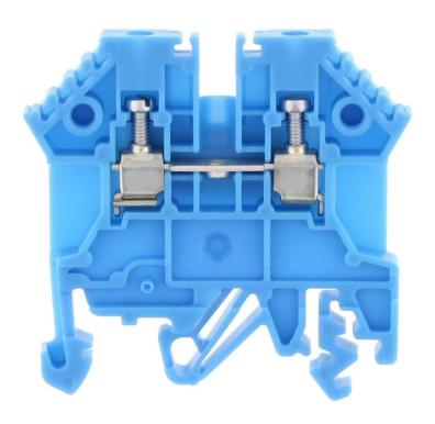
Feed-through terminal, Screw connection, Mounting type:Mounting rail TS 35/7.5, Rated cross-section: 2.5 mm², Width: 5 mm, Colour: Blue
