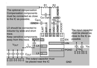
Figure 4. PCB Layout Guide
