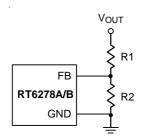
Figure 2. Output Voltage Setting
