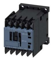
Power contactor, AC-3 7 A, 3 kW / 400 V 1 NO, 110 V AC, 50 Hz, 120 V 60 Hz, 3-pole, Size S00 ring cable lug connection
