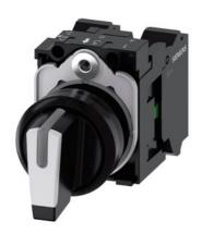
Selector switch, illuminable, 22 mm, round, plastic, white, selector switch, short, 3 switch positions I-O-II, latching, 10:30h/12h/13:30h, with holder, 1 NO, 1 NO, spring-type terminal, with laser labeling, lower case
