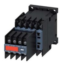
contactor relay, 4 NO + 4 NC, 48 V DC, size S00, ring cable lug connection, captive auxiliary switch
