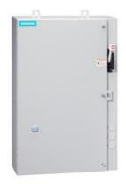
Non-reversing motor starter, Size 1, Three phase full voltage, Solid-state overload relay, OLR amp range 0.25-1A, Combination type, 30A fusible disconnect, 30A/600V fuse clip, Enclosure NEMA type 4/12, Water/dust tight for outdoors, Extra-wide enclosure
