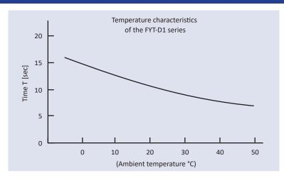
■ Damper characteristics vary according to the ambient temperature. In general, the damper characteristics become weaker as the temperature increases, and become stronger as the temperature decreases. This is because the viscosity of the oil inside the damper varies according to the temperature. When the temperature returns to normal, the damper characteristics will return to normal as well. The changes in the time it takes for the lid to close are shown in the graph to the left.
