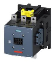
Power contactor, AC-3 400 A, 200 kW / 400 V Coil AC 50/60 Hz and DC 200-277 V x (0.8-1.1) F-SPS input 24 V DC 3-pole size S12 Auxiliary contacts 2 NO + 2 NC permanently mounted Main circuit: Busbar Control and auxiliary circuit: Screw terminal
