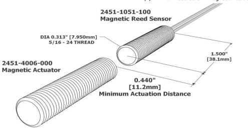
All measurements are in Inches [millimeters]
