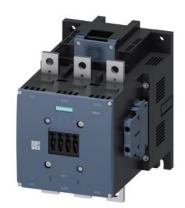
Power contactor, AC-3 500 A, 250 kW / 400 V AC (50-60 Hz) / DC 23-26 V AC / DC Auxiliary contacts 2 NO + 2 NC 3-pole, size S12 Busbar connections Operating mechanism: conventional screw terminals NEMA version
