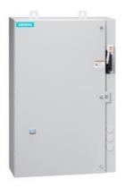
Non-reversing motor starter, Size 1, Three phase full voltage, Solid-state overload relay, OLR amp range 0.25-1A, Combination type, 30A fusible disconnect, 30A/600V fuse clip, Encl NEMA type 4X 304 S-Steel, Water/dust tight noncorrosive, Extra-wide enclosure
