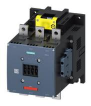
Power contactor, AC-3 400 A, 200 kW / 400 V Coil AC 50/60 Hz and DC 96-127 V x (0.8-1.1) F-SPS input 24 V DC 3-pole size S12 Auxiliary contacts 2 NO + 2 NC permanently mounted Main circuit: Busbar Control and auxiliary circuit: Screw terminal
