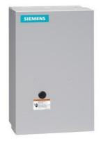
Electrically held lighting contactor, Contactor amp rating 30A, 0 N.C. / 6 N.O. Poles, 24VAC 50/60HZ coil, Non-combination type, (no disconnect device), Enclosure NEMA type 1, Indoor general purpose use
