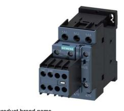
Power contactor, AC-3 32 A, 15 kW / 400 V 2 NO + 2 NC, 220 V AC 50/60 Hz, 3-pole Size S0, screw terminals Removable auxiliary switch
