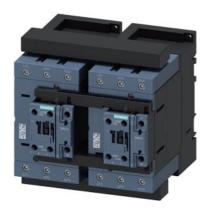
Reversing contactor assembly, AC-3, 45 kW 400 V, 20-33 V AC/DC 3-pole, Size S3 screw terminal electrical and mechanical interlock 2 NO and varistor integrated
