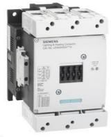
Electrically held lighting contactor, Contactor amp rating 400A, 0 N.C. / 3 N.O. Poles, 24VAC 50/60HZ coil, Non-combination type, (no disconnect device), Enclosure NEMA type (open), No enclosure
