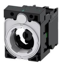
holder, 3-way, plastic, 1 NO, LED module, blue, 6-24 V AC/DC, screw terminal  $\,$
