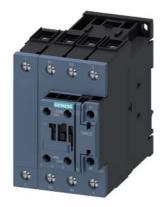
Contactor, AC-3, 22 kW/400 V 110 V AC/50 Hz/120 V AC/60 Hz 4-pole, 2 NO+2 NC, Size S2 Screw terminal 1 NO+1 NC integrated
