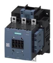
power contactor, AC-3 185 A, 90 kW / 400 V AC (50-60 Hz) / DC operation 23-26 V AC/DC auxiliary contacts 2 NO + 2 NC 3-pole, frame size S6 busbar connections drive: conventional spring-loaded terminal
