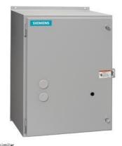
Electrically held lighting contactor, Contactor amp rating 200A, 0 N.C. / 3 N.O. Poles, 220VAC 50HZ/240VAC 60HZ coil, Non-combination type, (no disconnect device), Enclosure NEMA type 1, Indoor general purpose use
