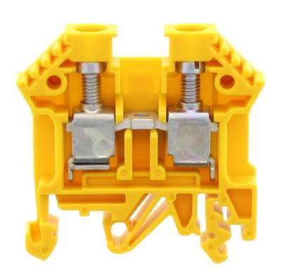
Feed-through terminal, Screw connection, Mounting type:Mounting rail TS 35/7.5 and TS 32, Rated cross-section: 10 mm², Width: 8 mm, Colour: Yellow
