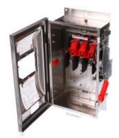
Siemens Low Voltage Circuit Protection Heavy Duty Safety Switches. Type: ENCLOSED, SAFETY SWITCH Std: UL V. Rating: 600V A. Rating: 60A No. Of Poles: 3P F. Rating: 60Hz Action: SINGLE THROW Material: SS Enclosure: TYPE 4X. 2-3 point mounting holes. Insulation: YES O. Cycles: 10000 O. Temperature: (-20F-120F) AMBIENT TEMPERATURE Environmental Conditions: INDUSTRIAL CORROSIVE RESISTANCE
