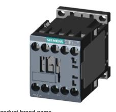
Power contactor, AC-3 16 A, 7.5 kW, 400 V 2 NO + 2 NC 220 V AC, 50 Hz, 240 V, 60 Hz 4-pole Size S00 Screw terminal
