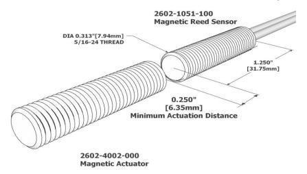
All measurements are in Inches [millimeters]
