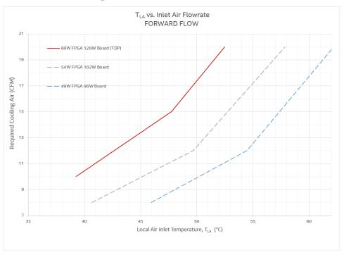
Table 11. Local Air Inlet Temperature and Air Flow Values for Forward Cooling Forward Flow Requirements to maintain FPGA  $T_j$ = 95 °C
