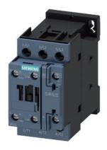
Power contactor, AC-3 32 A, 15 kW / 400 V 1 NO + 1 NC, 48 V AC 50/60 Hz, 3-pole size S0 screw terminals
