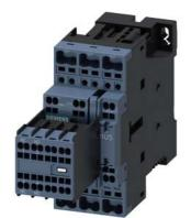
power contactor, AC-3 12 A, 5.5 kW / 400 V 2 NO + 2 NC, 110 V DC 3-pole, Size S0 Spring-type terminal Removable auxiliary switch
