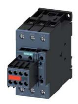
Power contactor, AC-3 80 A, 37 kW / 400 V 2 NO + 2 NC, 230 V AC 50 Hz 3-pole, size S2 screw terminals Perm. mounted auxiliary switch
