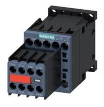
Power contactor, AC-3 12 A, 5.5 kW / 400 V 2 NO + 2 NC, 230 V AC, 50 / 60 Hz 3-pole, Size S00 Screw terminal Captive auxiliary switch
