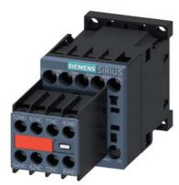
contactor relay, 6 NO + 2 NC, 220 V AC, 50 Hz, 240 V, 60 Hz, size S00, screw terminal, captive auxiliary switch
