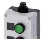
AS-Interface enclosure for command devices, 22 mm, round, Enclosure material plastic, enclosure top part gray, 2 control points plastic, Recess for labels, B=Pushbutton green, label: I, 1 NO, spring-type terminal, A=Pushbutton red, label: O, 1 NC, spring-type terminal, floor mounting, Insulation displacement system on top, Labels enclosed
