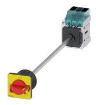
Load disconnector 3LD3, lu 32 A Main switch 3-pole Rated operating capacity for AC-23 A at 400V 11.5kW floor mounting Basic switch with door coupling Central hole mounting 22.5mm Toggle drive red / yellow 48x48 mm with auxiliary switch 10E + 1S
