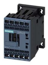
power contactor, AC-3 12 A,  $5.5\,\mathrm{kW}$  / 400 V 1 NC, 24 V DC 0.7-1.25\*US with integrated suppressor diode 3-pole, size S00 spring-type terminal suitable for PLC outputs not expandable with auxiliary switch
