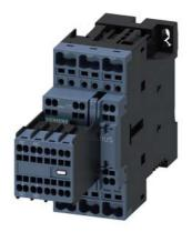
Power contactor, AC-3 38 A, 18.5 kW / 400 V 2 NO + 2 NC, 24 V DC 3-pole, size S0 Spring-type terminals Removable auxiliary switch
