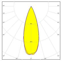
Dimensions: 37.5 mm x 37.5 mm Height: 24.17 mm ~35° wide beam with holder
