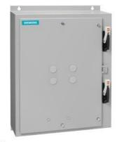
Duplex starter w/o alternator Size 1 Three phase full voltage Solid-state overload relay OLR amp range 3-12A 110VAC 50Hz / 120VAC 60Hz Coil Combination type Two 30A disconnect switches Encl NEMA type 4X 304 S. Steel Water/dust tight non-corrosive
