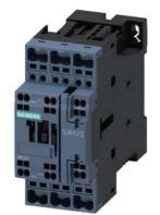
power contactor, AC-3 32 A, 15 kW / 400 V 1 NO + 1 NC, 24 V DC with integrated varistor 3-pole, size S0 spring-type terminal suitable for PLC outputs not expandable with auxiliary switch
