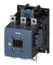
power contactor, AC-3 300 A, 160 kW / 400 V, AC (50-60 Hz) / DC operation 200-277 V AC/DC auxiliary contacts 2 NO + 2 NC 3-pole, frame size S10 busbar connections drive: electronic with PLC interface 24 V DC screw terminal
