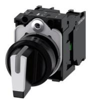
Selector switch, illuminable, 22 mm, round, plastic, white, selector switch, short, 3 switch positions I>O<II, momentary contact type, 10:30h/12h/13:30h, with holder, 1 NO, 1 NO, screw terminal, with laser labeling, upper case
