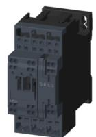
power contactor, AC-3 12 A, 5.5 kW / 400 V 1 NO + 1 NC, 110 V AC, 50 Hz 3-pole, Size S0 Spring-type terminal
