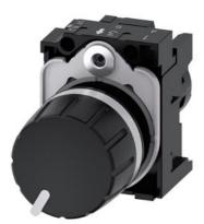
Potentiometer, compact, 22 mm, round, plastic, black, 1k ohm, with holder, screw terminal, with laser labeling, inscription or symbol Customer-specific selection with SIRIUS ACT configurator (CIN)
