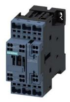
Power contactor, AC-3 38 A, 18.5 kW / 400 V 1 NO + 1 NC AC (50 - 60 Hz) / DC 95-130 V AC / DC, 3-pole Size S0, Spring-type terminals
