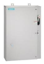
Non-reversing motor starter, Size 3, Three phase full voltage, Solid-state overload relay, OLR amp range 25-100A, 208VAC 60Hz coil, Combination type, 100A fusible disconnect, 100A/250V fuse clip, Encl NEMA type 4X 304 S-Steel, Water/dust tight noncorrosive, Extra-wide enclosure
