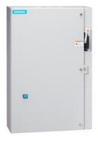
Non-reversing motor starter, Size 3, Three phase full voltage, Solid-state overload relay, OLR amp range 25-100A, 110V 50Hz / 120V 60Hz coil, Combination type, 100A non-fusible disconnect, Enclosure NEMA type 1, Indoor general purpose use, Extra-wide enclosure
