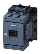
power contactor, AC-3 115 A, 55 kW / 400 V AC (50-60 Hz) / DC operation 440-480 V AC/DC auxiliary switch right 3RH1921-2DE11, 3-pole, frame size S6, with box terminals drive: conventional screw connection coil
