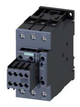
power contactor, AC-3 51 A, 22 kW / 400 V 2 NO + 2 NC, 48 V AC, 50 Hz, 3-pole, size S2, screw terminal
