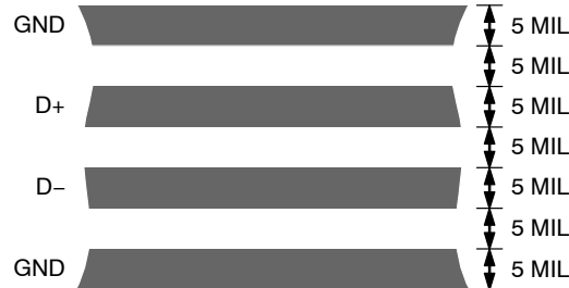
Figure 28. Arrangement of Signal Tracks
