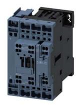
Power contactor, AC-3 25 A, 11 kW / 400 V 2 NO + 2 NC 220 V DC, 50 Hz 240 V, 60Hz, 1 NO + 1 NC 4-pole size S0 Spring-type terminals 1 NO + 1 NC integrated
